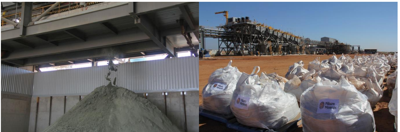
Above: Fines concentrate production from filter press (left hand side) and tantalite product bags (right hand side) ready for delivery
