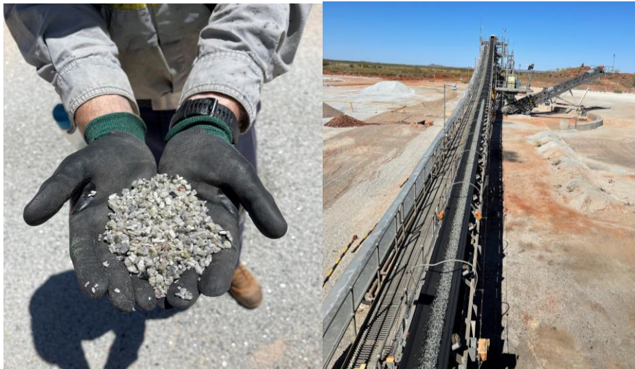
Above: First concentrate from the coarse production circuit of the Ngungaju Plant
