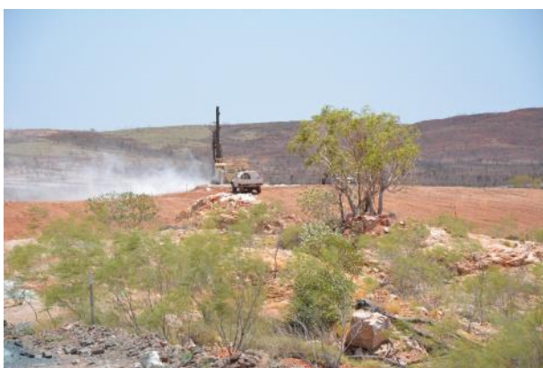
Grade control and blast drilling underway at Tabba Tabba
