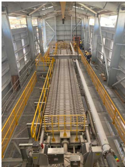
Above: New concentrate filter press and filtered product.
