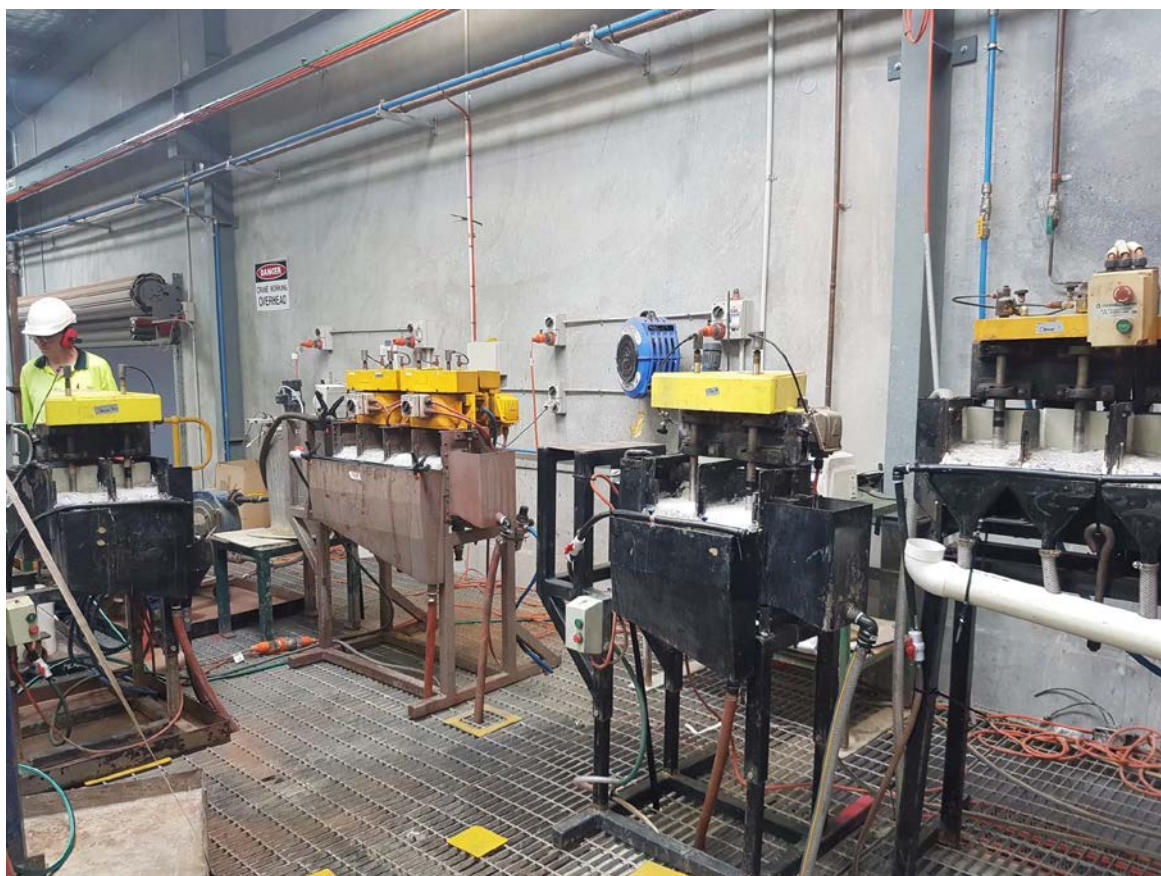
Figure 2: Flotation Pilot Plant – Commissioning on Bulk Eastern
