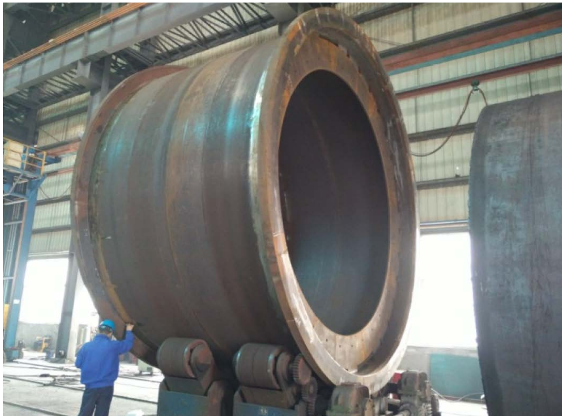
Figure 7: Ball Mill – Mill shell section
