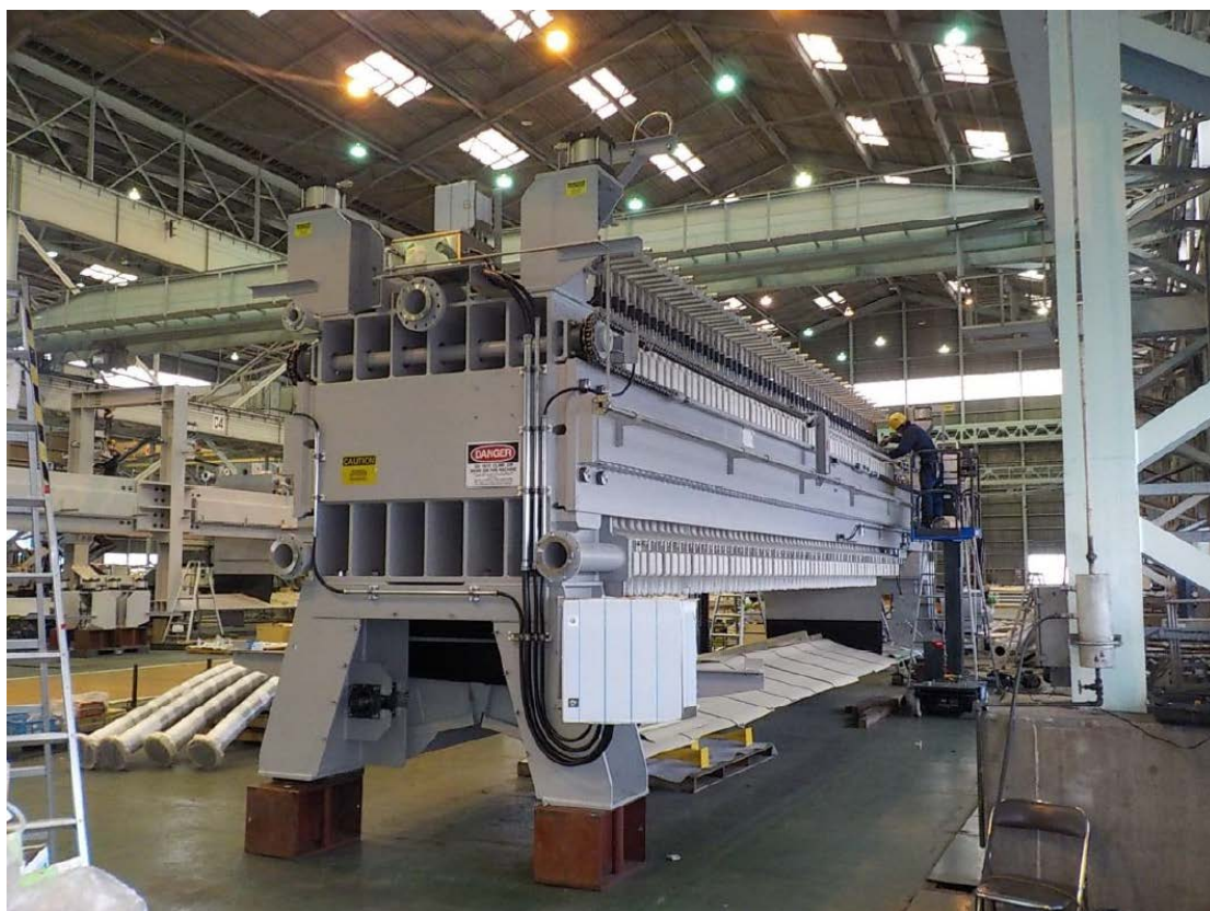
Figure 4: Concentrate Filter Press.
