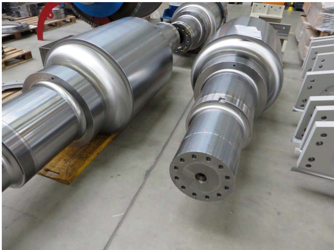
Figure 6: HPGR – Tyre shafts
